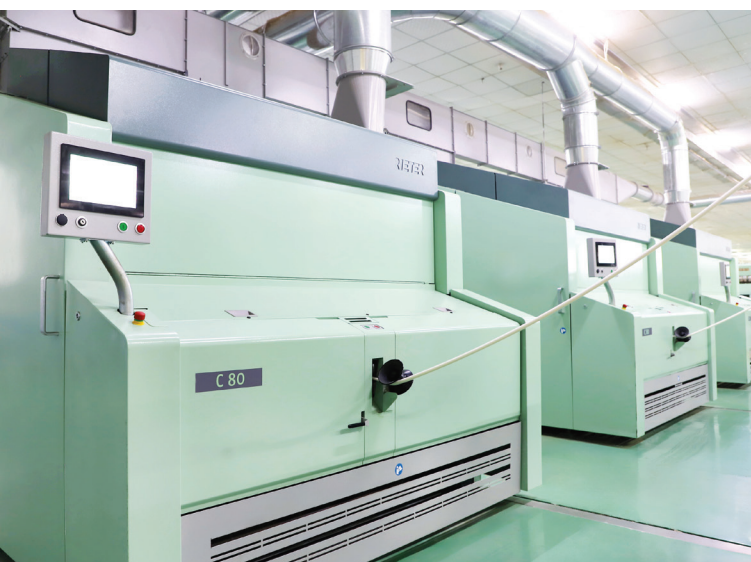
Figure 1: The C 80 produces up to 120 kg/h, far exceeding the output of previous models.
